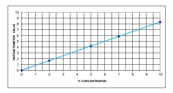
The data provided for the % concentration control is prepared according to the data obtained for the freshly prepared emulsion. As the utilization time of the emulsion and the undesired oil/contamination amount in the system increases, deviations from the data stated above should be taken into account.
