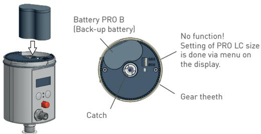
Insert the battery PRO B into the drive unit (according to the direction of the arrow on the label).
