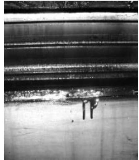
Fig. 42: Load-carrying pattern after ten operating hours with a running-in lubricant
