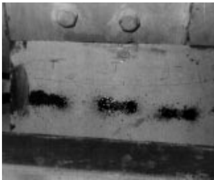
Fig. 27: Inadequate spray patterns; the individual patterns do not overlap
