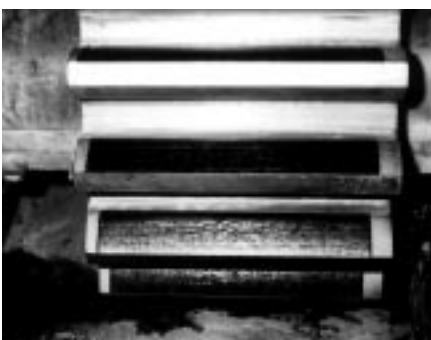
Fig. 41: Contact ratio/load-carrying pattern made visible by means of priming lubricant
