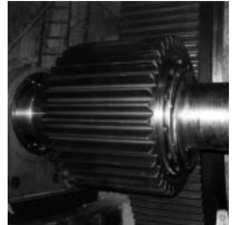
Fig. 5: Gear drive with tiltable pinions during assembly (Krupp-Polysius)
