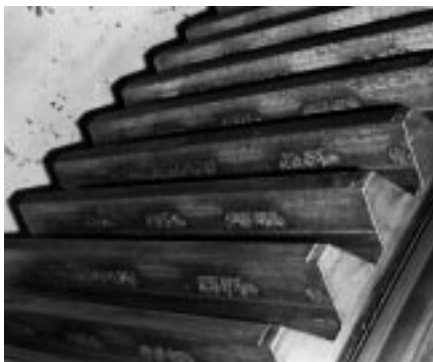
Fig. 28: Scuffing caused by partially insufficient lubrication (individual spray patterns do not overlap)
