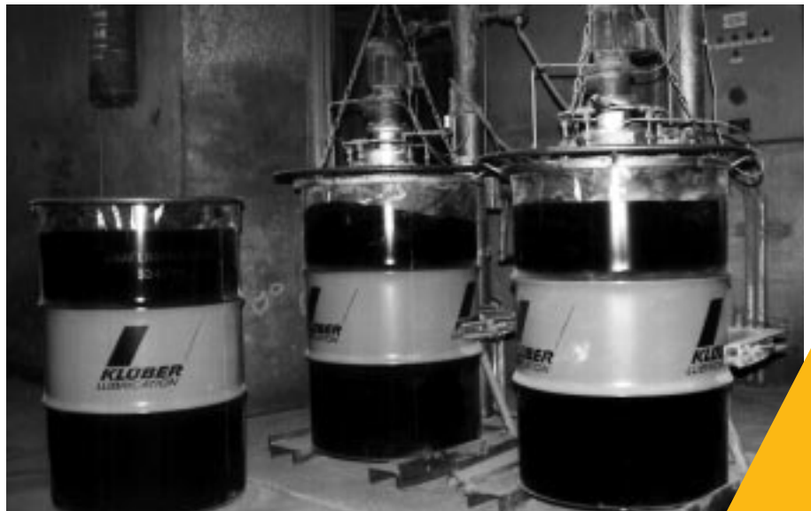
Fig. 36: Original lubricant drums from Klüber Lubrication with flexible internal liners and mounted barrel pumps
