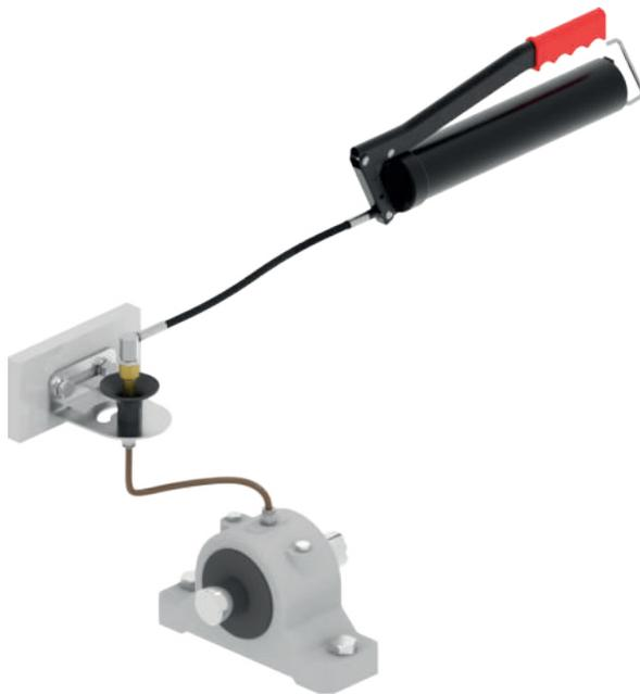
6. Use a tube prefill adapter to prefill lubrication point and grease lines:
