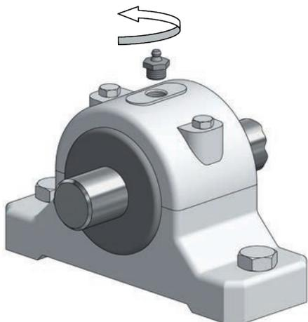
Determine thread size at the lubrication point with perma fitting thread tester **Art. No. 110374**
