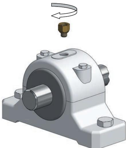
4. Lubrication point, accessory parts and tubes / hoses must be pre-filled with lubricant.
