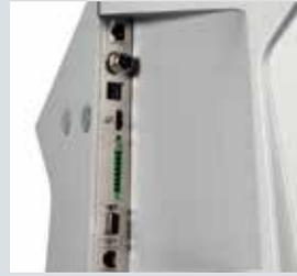
The PHOENIX offers all the necessary connections for accessories including the sniffer line or the partial flow system. Furthermore, it has easily accessible USB ports and additional controlling interfaces.
